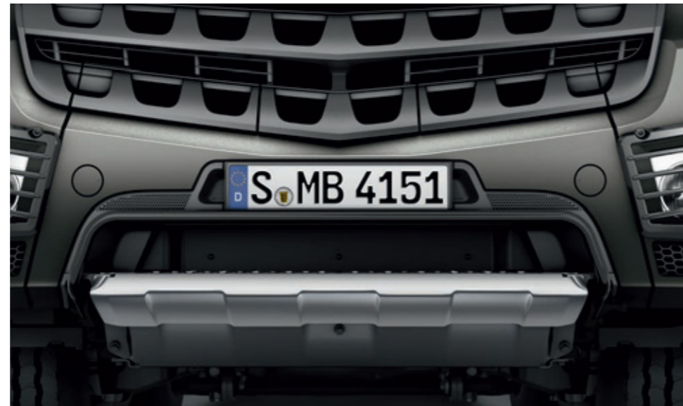
Protective plate for engine and radiator. Many off-road models come with a steel plate to protect the radiator and the engine.
